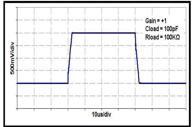
Large-Signal Step Response, 2V Step
