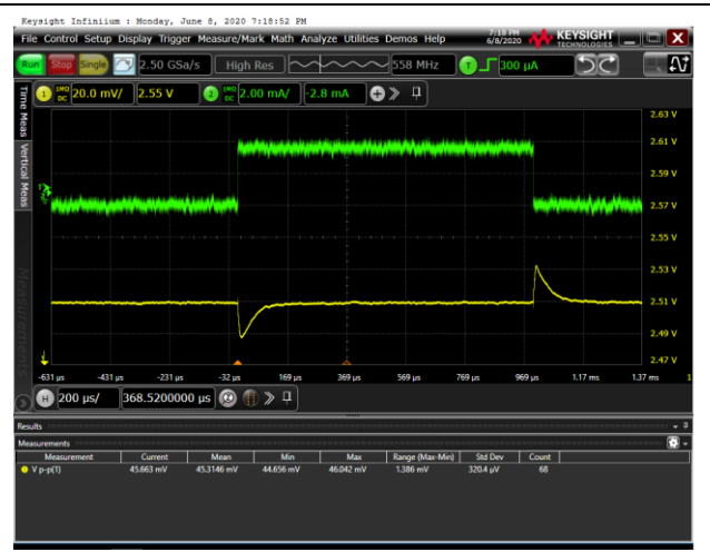
Figure 14. Load Transient, \pm 2 mA, V_{IN} = 2.8 V, C_{IN} = 1 \mu\text{F} , C_{OUT} = 1 \mu\text{F} , 20 mV/div
