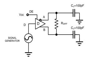
Figure 2A. Test Circuit
