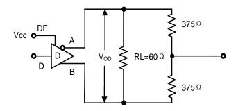
Figure 1B. VOD with Common Mode Load
